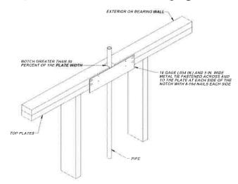
\*\*Figure R602.6.1; delete the figure and insert the following figure:
